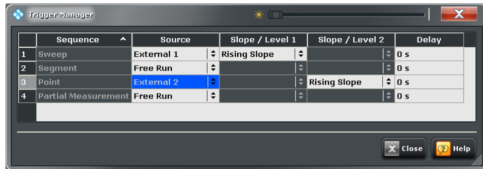
Figure 4-10: Example of a multiple trigger configuration
